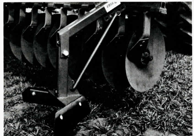
V-shaped blade is adjustable for height and pitch.
