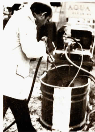
Paul Gerber demonstrates cold water washer which delivers up to 5 gal. per min. at up to 2,000 psi.
