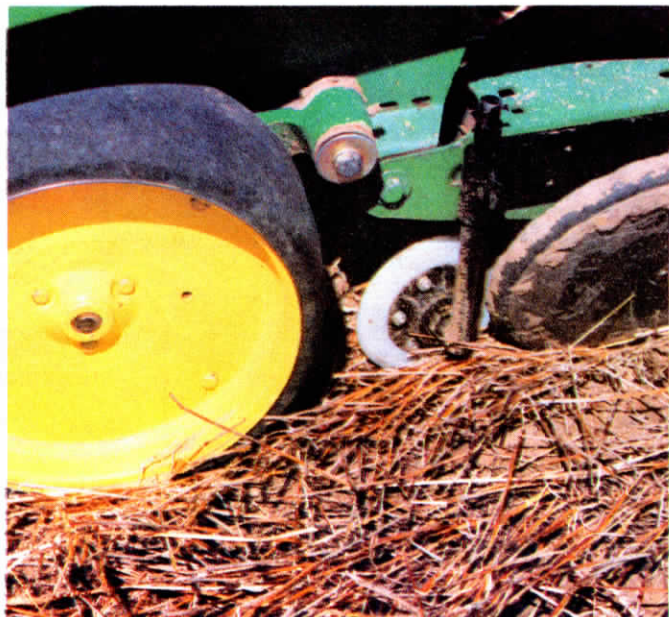
Schaffert's 5 1/2-in. dia. poly wheel sets between disc openers and closing wheels and runs 3/4 to 1 in. off to side of furrow.
