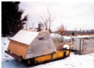
Pigott stripped two snowmobiles down and welded the frames together side by side to pull heavier loads out of the woods.
