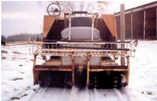
With no skis to catch on brush and a steel bumper with an angled skid plate that Pigott made for the front end, the Doo Doo will go right over most low growing brush and even walk over the top of a 7-in. log on the ground.
