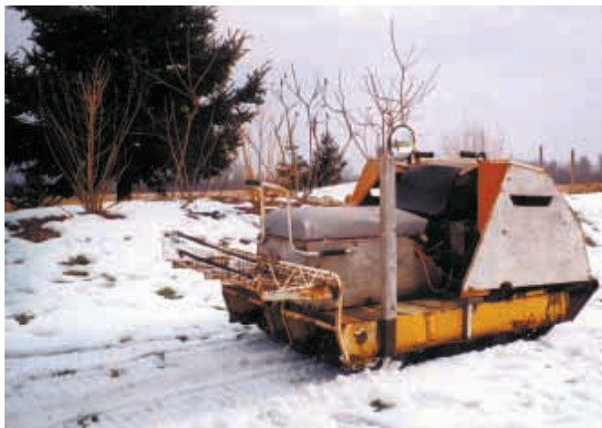
After remounting engine, Pigott added a jackshaft with a pulley at both ends. A belt from engine powers jackshaft. Belts from each of the end pulleys drive the individual tracks.
