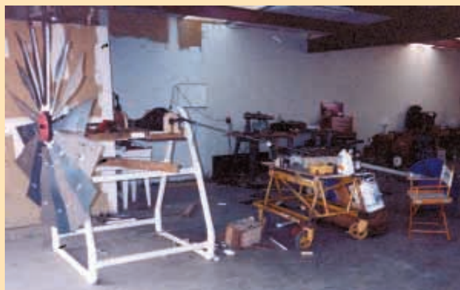
Love's home-built, portable windmill is shown here set up for well pump application. It mounts on a frame made from pvc pipe.
