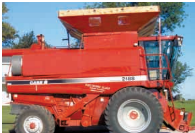
Patent pending electronic scale is built into the body of Steve Kaltenheuser's Case-IH 2188 combine. Weigh bars attach to combine's front axle and spindles on rear axle.
