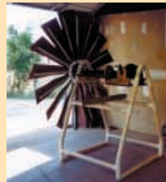
Love's home-built, portable windmill is shown here set up for well pump application. It mounts on a frame made from pvc pipe.
