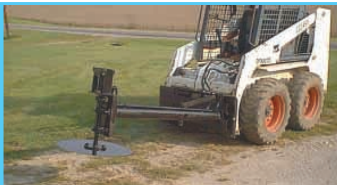
Bobcat-mounted brush-cutting saw measures 26 1/2 in. in diameter and is equipped with carbide teeth.
