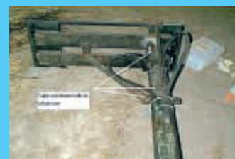
Hydraulic motor direct-drives shaft, connected by a chain coupler to a steel plate (left). By removing three bolts from mounting plate, Boyd can manually rotate saw blade to a vertical position.
