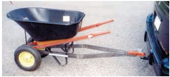
Rodger Aanderud used two lengths of steel tubing to make a diamond-shaped hitch with a ball hitch at one end. It makes hauling dirt in his wheelbarrow easier.
