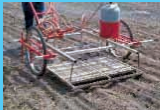
Flat panel flamer has two burners. Attachments for spraying, seeding and cultivating are also available.
