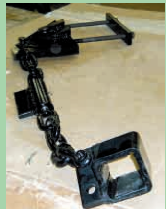
An old Allis Chalmers tractor gave Nebgen the idea for this device that stabilizes Deere hitches.
