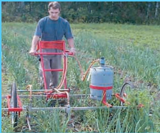
Petri Leinonen says you can cover up to 5 acres per day using the Weed Master, which has wide steering handles and a waist-high web belt that the operator walks into to push it through the field.
