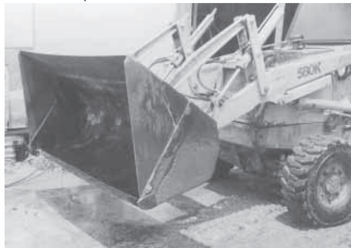
Dale Johnson added capacity to his loader bucket by adding sheet metal to the sides and back. "It was a lot cheaper to modify the bucket than to buy a new one," he says.
