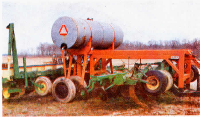
The Wolfs plant at 4.5 to 5 mph with their "one pass" implement carrier which allows a once-over till-plant-spray operation.
