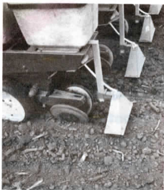
Hinged hoods let you band chemicals without worrying about wind or obstacles on the ground.
