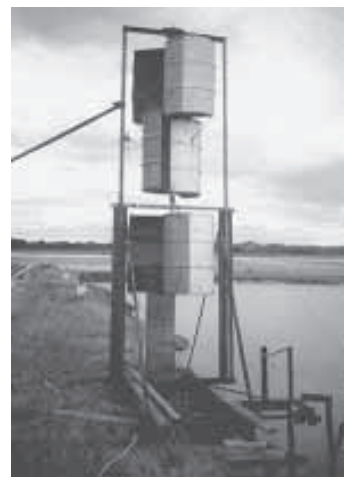
Windmill is made from steel barrels that drive an old car rear end, which serves as a right angle drive to power a conventional windmill piston pump.
