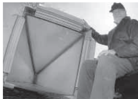
Fred Brammeier says his windmill, which is shaped like a pyramid laying on its side, works on the same principle as an airplane wing. When air hits the point it's forced up the slanted sides. Note turbines on three sides of the base.
