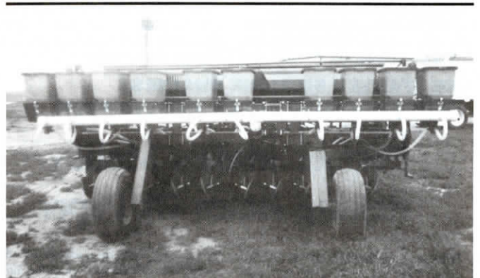
Seed is delivered to drill's rear gang by special-designed Crary air system modified to adapt to conventional Max-Emerge planter boxes.
