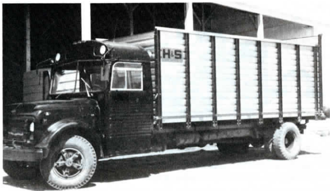
Kinnard mounted 24-ft. rear unloading silage box on 1973 GMC 72-passenger bus.
