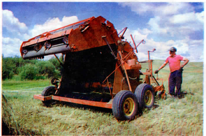
Hydraulic bypass cylinder on ejector door is used to adjust bale tension.
