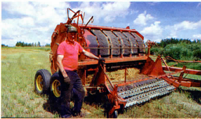
Baler has six belts that are bolted together instead of laced to make repairs easier.
