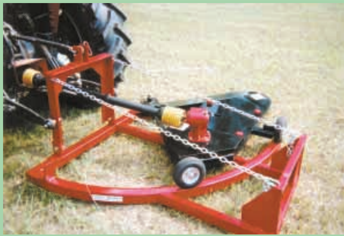
“Fence Mower” deck swings back and forth on a pair of wheels on a curved steel track. It automatically glides around fence posts and other obstacles.
