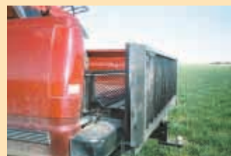
Hinge mechanism allows ramp to fold up neatly behind box.
