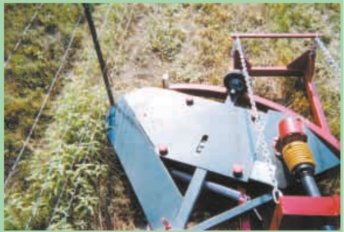
Rototiller-type spade works with mower blade to knock down mounded dirt under fence lines.
