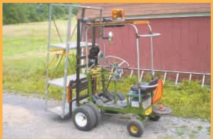
Home-built electric forklift is powered by two 12-volt deep cycle batteries that run for several hours on one charge.
