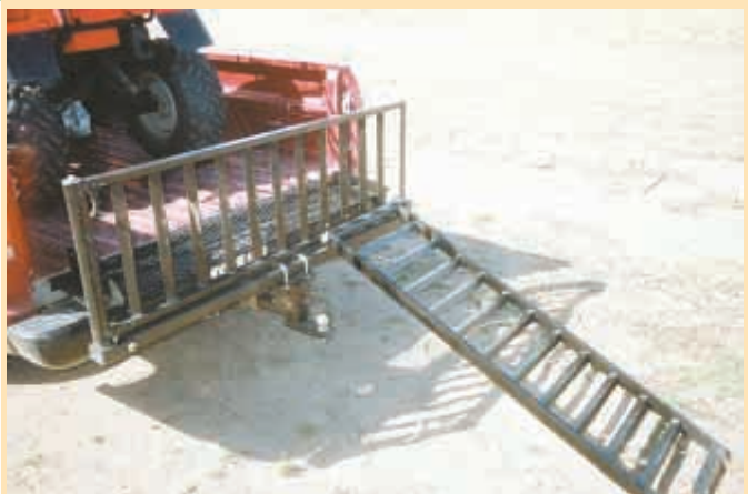
Ramp assembly fits into receiver hitch. When needed, ramps fold out for loading without ever detaching from pickup.
