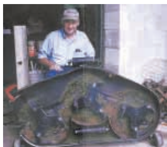
Only the knives will ever have to be replaced, unlike conventional single blades where you have to replace the whole thing, notes Murray.
