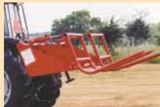
Hay Handler can be fitted with either bale spears or twin forks.
