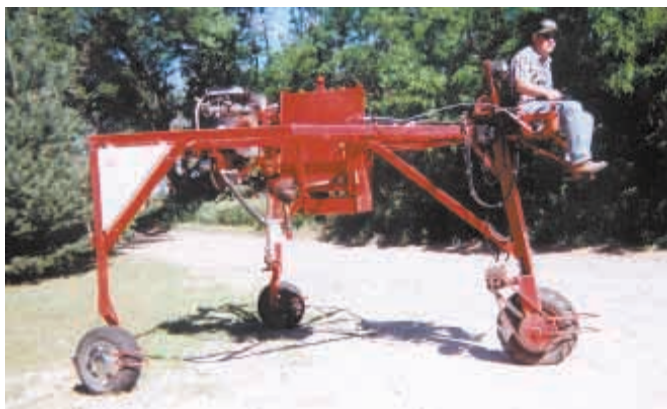
"It lets me drive through the field without knocking down any of the crop," says Terry Kuchera about his high clearance "field checker".
