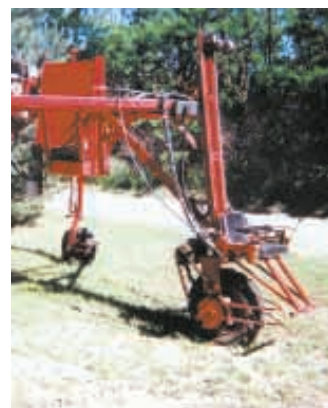
Driver's seat moves up and down column above the front wheel, powered by an electric winch that operates off the engine's battery.
