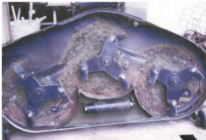
To save money on the cost of new replacement blades, Walter Murray came up with cutting discs fitted with three swivel-mounted blades.
