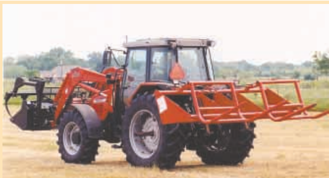
Independent hydraulic cylinders on each side of the Hay Handler let you pick up and drop bales one at a time.
