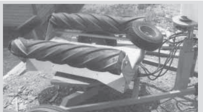
A front-end loader is used to load bales onto a pair of rubber rollers that came off a New Holland haybine.
