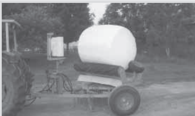
Using parts from several old machines, Chris Ross built his own pull-type round bale wrapper entirely from scratch. The controls mount on the machine's tongue.
