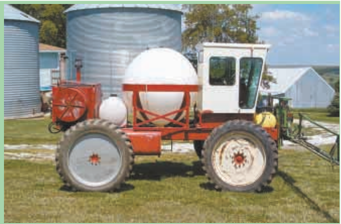
With a 120-in. tread width and 118-in. wheelbase, sprayer is stable on side hills.
