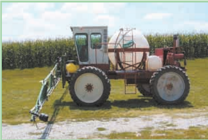
Dale Huneke's sprayer is fitted with a 750-gal. spherical tank, which makes it easy to clean out.
