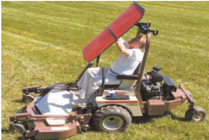
Operator can remove lightweight canopy without ever leaving his seat.
