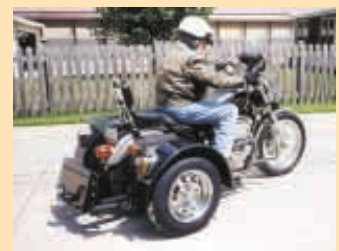
Voyager conversion kit adds two wheels to motorcycle, which stabilizes ride but still lets you lean on turns.
