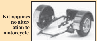
Voyager conversion kit adds two wheels to motorcycle, which stabilizes ride but still lets you lean on turns.
