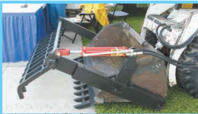
Attachment uses pivoting "fingers" to pull rocks into bucket.
