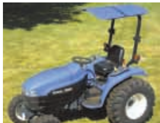
Canopy is made from modular, nearly indestructible thermoplastic panels.
