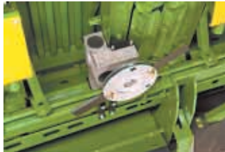
System features one gearbox unit per row with two rotary chopper knives. Knives can be easily removed if chopping is not desired.
