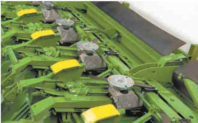
StalkMaster chopper is designed for use on 8-row, 30-in. and 12-row, 22-in. corn heads.
