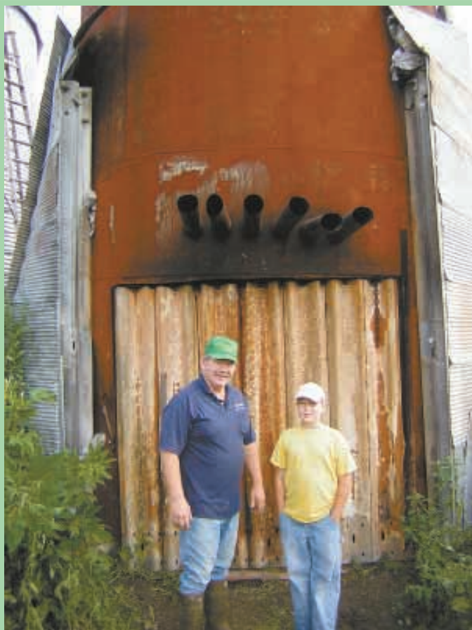
Craig Stortz cut his corn drying cost by more than half last year using this bean residue burner. The burner preheats air going into his crop dryer.
