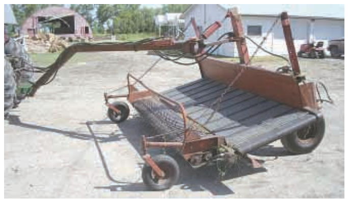
Leroy Groening's home-built hydroswinging swath turner works much like a commercial hydroswinging mower - except that instead of mowing hay it turns the swath over.
