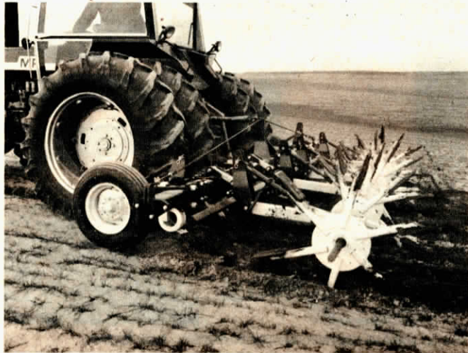
Diker digs holes 5 in. deep, 6 in. in dia., and spaced 2 ft. apart to trap water.
