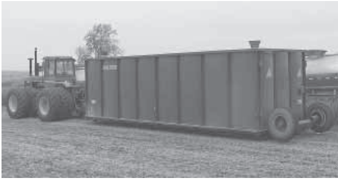
Big 17,500-gal. tank is designed to be parked in the field where semi trucks can load it with manure. A pto-driven pump on front can be used to load and unload.
