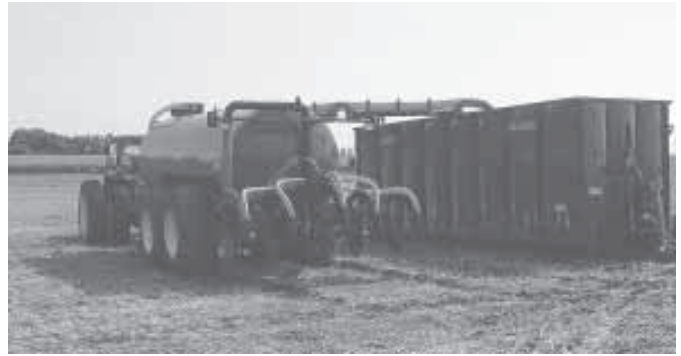
A Balzer vacuum boom tank draws a load from the field storage unit. Load time is 3 to 4 minutes using an 8-in. load hose or tube.
