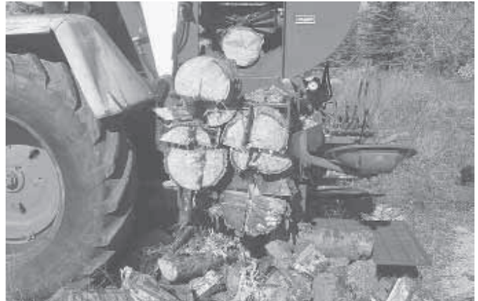
A manually-operated splitter pushes log through 10-way grate with 50 tons of force.
