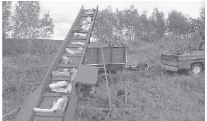
A 30-ft. elevator carries wood up into trucks, wagons or wood piles.
