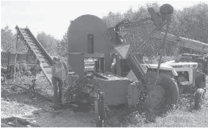
Tongs pull log up to processor where hydraulic-driven rollers feed it into blade opener.
