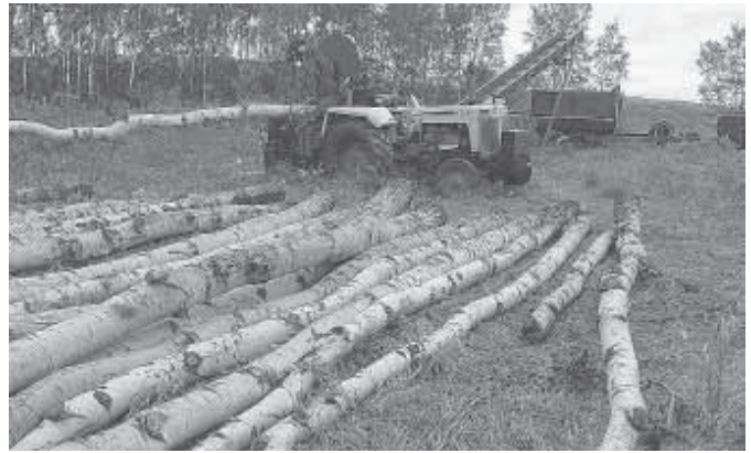
Rollers hold log up in the air as it's fed into processor. No log table is needed.
