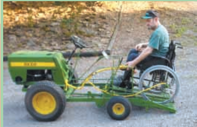
Bragdon uses a long lever to lower the bed to the ground. Electric winches pull the ramp and wheelchair up onto the tractor.
