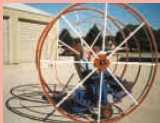
"Car" steers like a skid steer. The wheels ride between two different size rings, one above the other.
