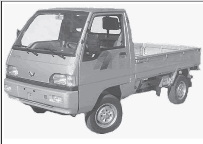
Chinese-built mini trucks are easy to work on because the seats tilt up for easy access to the engine.
