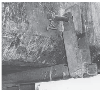
Rear bracket pins to metal hitch welded to back side of bucket.
