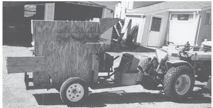
Orville Hillis's home-built thresher consists of a 4 by 4-ft. by 15-in. wide plywood shell fitted with two cylinders, a concave and a cleaning sieve.
