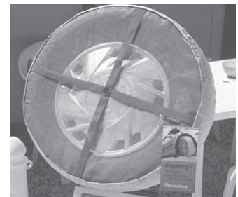
Autosocks are lightweight elastic fabric coverings for car and truck tires. You just slip them over your tires and drive off. They're inexpensive, machine washable and reusable.
