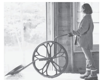
Wovel is made from lightweight steel and plastic. The shovel mounts ahead of the 3-ft. dia. wheel. Handle pivots on the wheel axle. This turns the unit into a lever which requires half as much the operator effort.
