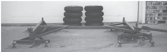
Skis are made from 1/4-in. thick flat steel and measure 2 in. wide by 1 ft. long. "The skis let you use the wagon during the winter for hauling firewood or taking wild game out of the woods, or just giving your kids a ride," says Wilbert Sas.
