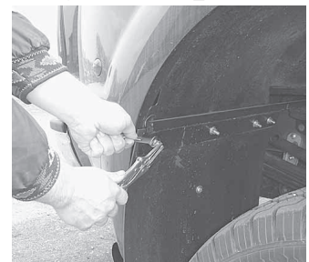
Bracket extends the width of the pickup. "You don't have to drill any holes in the pickup body at all," says Mace Kanten.
