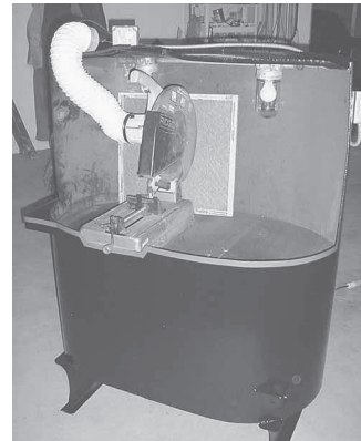
Chop saw cabinet was made from a 275-gal. fuel oil tank. It catches fines, traps sparks and provides an easy-to-clean work surface.
