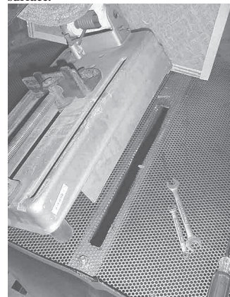
Work table is made from perforated metal screening. Fines blow through the perforations. A slot beneath the saw lets large chunks fall straight through.
