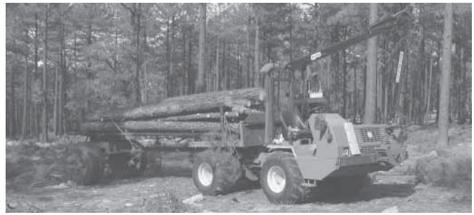
West found a Komatsu articulated dump truck, put a knuckle boom on it, took the sides off, and turned the bed into a log trailer.
