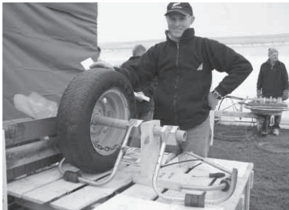
Trailer walker can be fitted and removed in seconds. It works by progressively chocking the trailer wheels as the drawbar is levered from side to side, which makes it easy to push or pull a trailer even if it’s heavily loaded.
