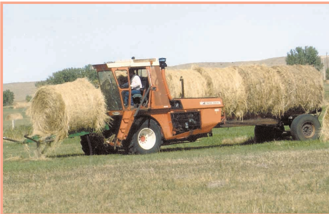
“Everyone thought I was crazy to build it, but it worked out just fine,” says Tom Davis, who attached a 38-ft. long, self-loading trailer to a New Idea Uni-Harvester power unit.
