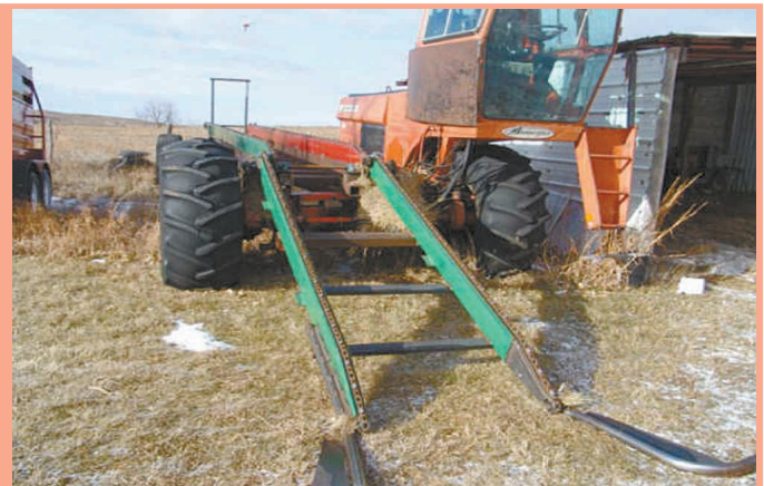
Chain conveyor on loading arm delivers bales onto trailer, which is also equipped with a chain conveyor.
