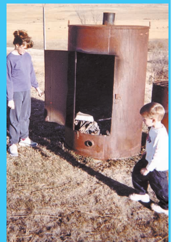
Tom Strasburger converted an old 300-gal. fuel oil tank into this enclosed garbage burner.
