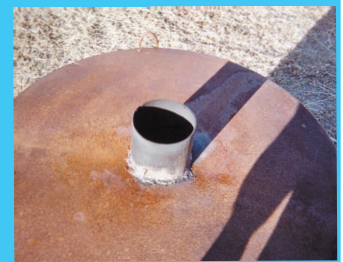
Tank has a chimney on top and drafts from the bottom for a fast burn.
