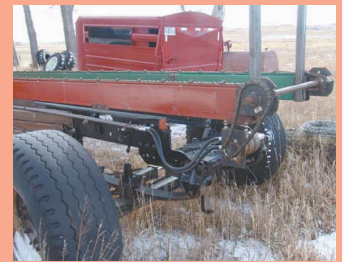
Davis made trailer’s steering axle by cutting the steering axle and wheels off an old semi tractor.
