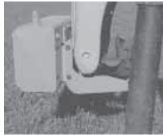
Unit looks like front-mounted tractor weights but adds less than 150 lbs. to the front of the tractor. Drain plug is at the bottom left and recessed for protection (right).
