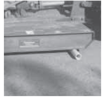
Tiller hangs from shed roof on a chain sling (left). To move crop shredder around, Loyd puts a short piece of pvc pipe under each side of the front part of the shredder.
