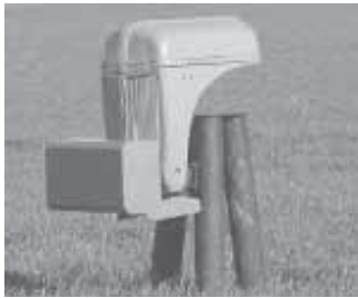
Unit looks like front-mounted tractor weights but adds less than 150 lbs. to the front of the tractor. Drain plug is at the bottom left and recessed for protection (right).
