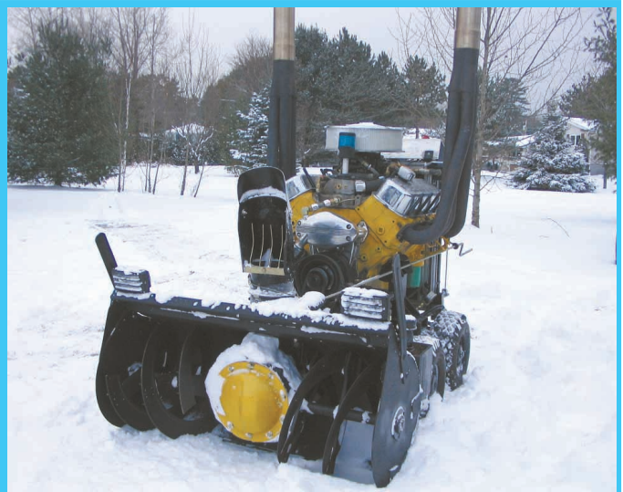
Big snowblower is powered by a Chevy 454 cu. in., V-8 gas engine producing 412 hp.
