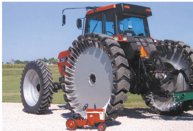
Steve Kaltenheuser says putting Tall Wheels on his tractor lets him cover ground faster than he could with his self-propelled high clearance sprayer.
