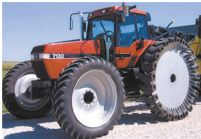
He built his own 8-ft. high rear wheels and uses bolt-on tire lugs on them.
