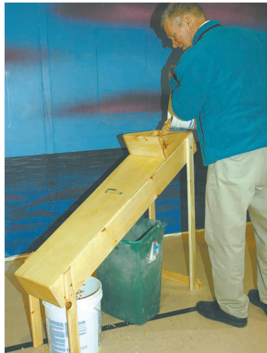
Dirty corn is poured into top opening. Clean corn falls into bucket at bottom. Middle container catches screenings that fall through.
