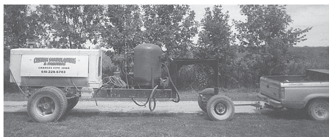
Jeff Hobert made his own sand blaster using the frame off a 3-ton grain truck and a 120-gal. LP tank.
