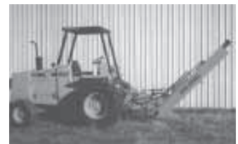
Pivot mount option makes it easy to set posts at an angle.
