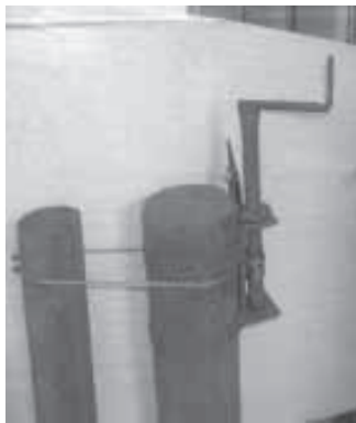
Winch-type gate closer mounts on top of any post.
