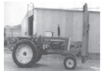
Heavy duty post driver can also be mounted on a tractor.
