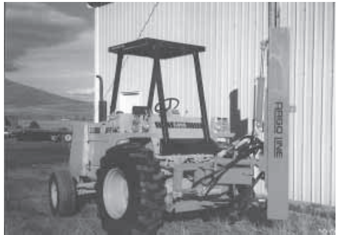
Arthur Argo's post-driving hammer weighs 1,000 lbs. and has an impact force of 114,000 lbs. He likes using it on a "rough-terrain" forklift.
