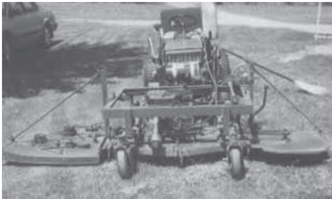
A 12 1/2 hp Briggs & Stratton engine powers three decks that cut a 100-in. swath at a time. Side decks fold up when not used.
