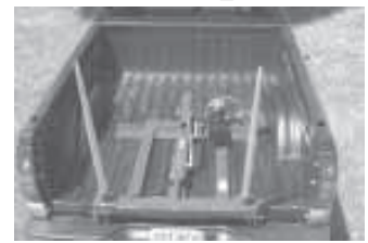
Pivoting bale spears on a steel frame mount to truck bed or attach to gooseneck hitch.
