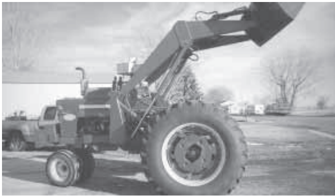
George Buseman, Jr. reversed a 560 IH LP tractor, putting a Koyker K-5 loader on it that faces backwards.
