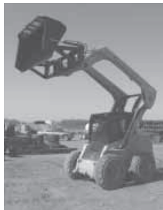
Bucket lets operator reach farther into the center of a truck or wagon when dumping.
