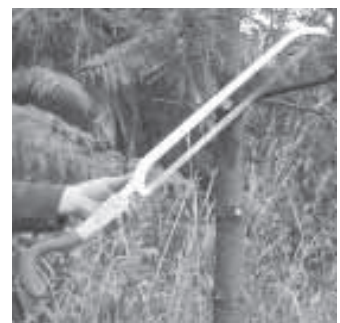
The secret to Havel's new handsaw is its length, weight and hook tooth bandsaw-type blades.
