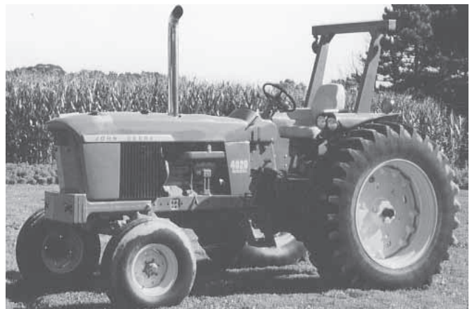
Tom Van Pelt replaced the original engine in his Deere 4020 tractor with a 466 cu. in. engine from a 7720 Deere combine.
