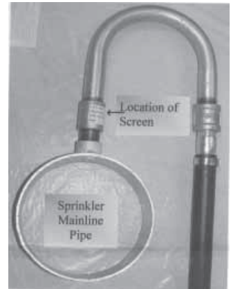
Coupler installs just above main line rather than down by the nozzle.
