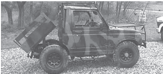
Al Wilson bought an old Samurai, cut off the rear end, and added a 4 by 3-ft. dump bed. He then gave it a paint job and replaced the wheels with 15-in., 12-ply tires off a forklift.
