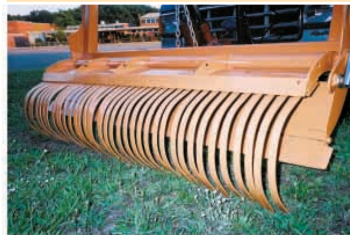
Claw-like truck attachment has a steel blade at bottom and curved rake tines on top that pivot up and down.
