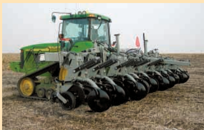
Hiniker recently introduced attachments for its 6000 Series cultivators that turn them into strip-tillage units. To cultivate normally, just unbolt the attachments and head back to the field.
