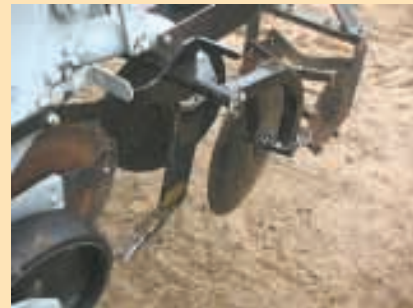
Hiniker recently introduced attachments for its 6000 Series cultivators that turn them into strip-tillage units. To cultivate normally, just unbolt the attachments and head back to the field.
