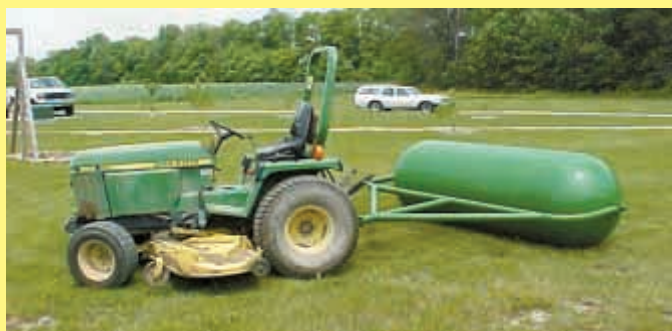
Joe Konecny used an old 3-ft. dia., 10-ft. long propane tank to make his lawn roller. "The rounded ends don't scuff the lawn when I turn," he points out.
