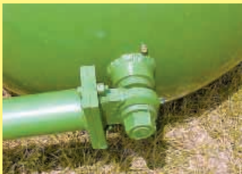
A friend made spindles for each end of tank. Bearings on tow bars slip over them.
