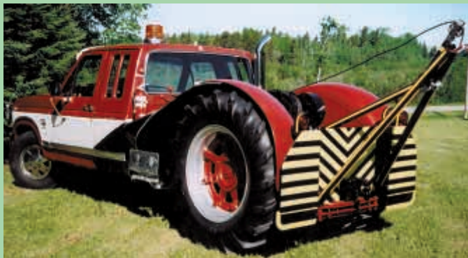
Back end of rig is equipped with a wrecker boom, pto and receiver hitch.
