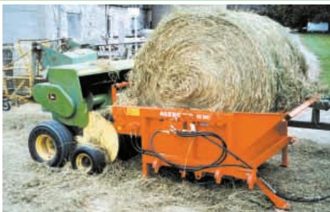
Machine unwinds bale directly over pickup reel of any small square baler. Here, a 4-ft. wide, 5-ft. dia. bale weighing about 800 lbs. is being unwound into a Deere 336.
