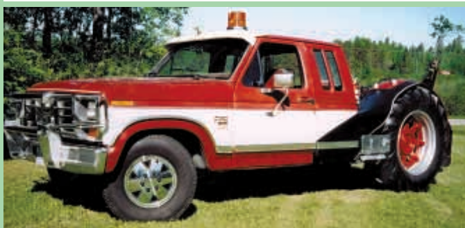
To build this truck-tor, Reg Crigger married a 1986 extended cab Ford F-150 1/2-ton pickup with the back end of a 1950 W-6 International farm tractor.
