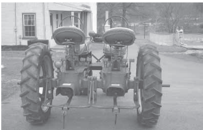
Evans says he had to cut the rear axle housing on each tractor, then weld them back together so they could be operated from either side.
