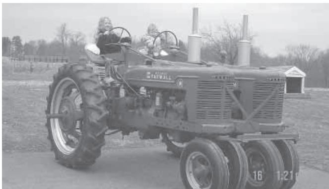
"Twinned Farmall H's" can be driven by one or both engines and have a clutch and transmission on each side.
