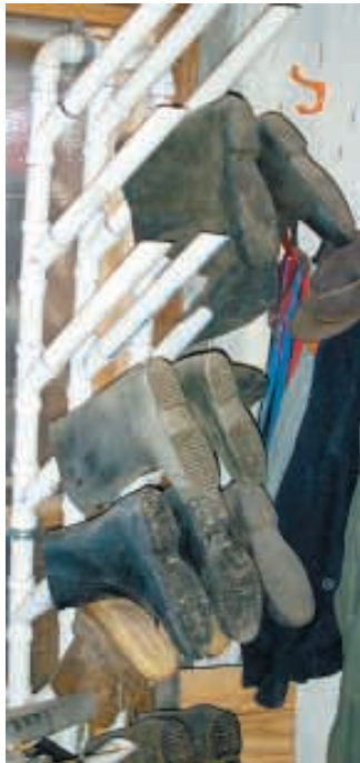
Andy Offenburger made this boot-drying rack from 1 1/2-in. pvc pipe. It mounts to the wall in his basement.
