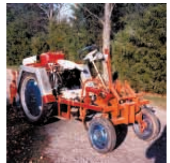
He took an Allis Chalmers WC two-row cultivator and remodeled it by putting one row in front and the other in back.
