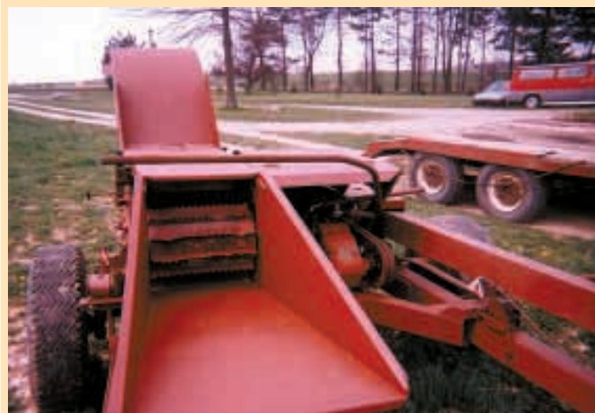
Eugene Keener turned a New Holland 717 forage harvester into this "chipper-chopper." A 3-ft. long, tapered chute extends out from the gathering rolls.
