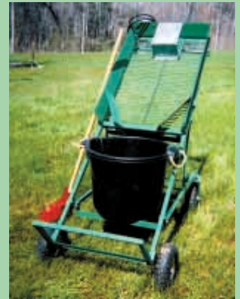
Electric bedding "recycler" consists of a 2 by 4-ft. metal screen set at an angle above a large plastic bucket. A 120-volt electric vibrator mounts at top of screen.
