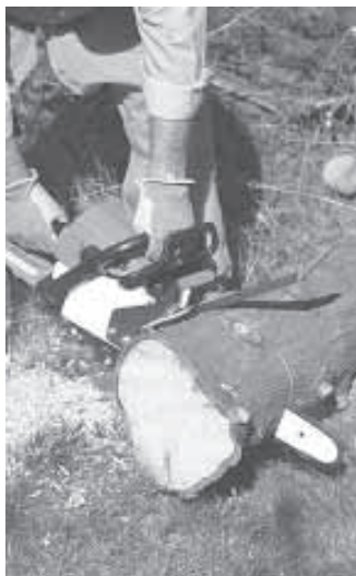
Guard doesn't prevent kickback but protects the operator from injury.
