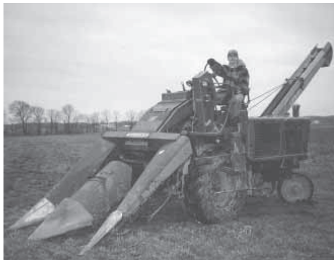
Corn picker consists of a late model 2-WD Minnesota Moline Uni-tractor's power unit, a New Idea husking bed, and an 83 Oliver 2-row picker snapping head.
