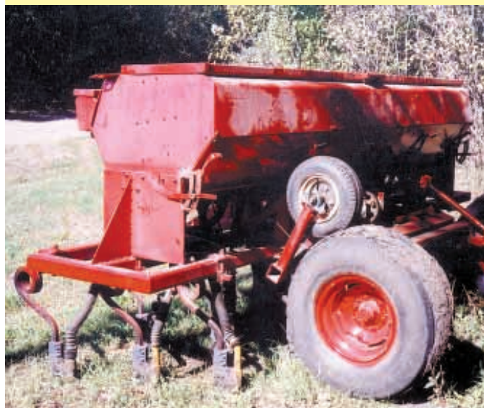
“I wanted something that could handle rough ground. It seeds right through rocky ground thanks to the Baker Boot shank openers on it,” says Scott Jones.
