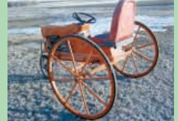
Tractor is fitted with three narrow wheels just 2 in. wide.
