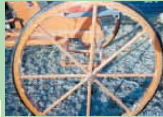
The 42-in. dia. rear wheels are covered with hard rubber.
