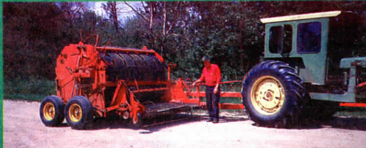
Inventor Joe Laczko with his built-from-scratch, offset baler that makes 8-ft. wide bales.
