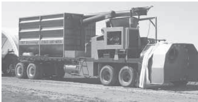
Self-contained unit has a 700-bu. surge tank. Its average capacity is between 1,200 and 1,500 bu./hr.
