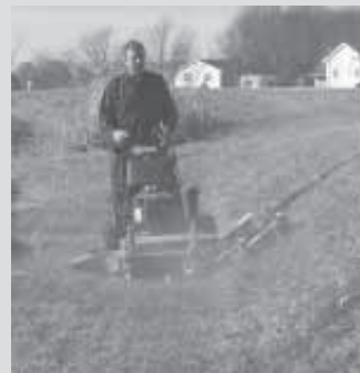
Flex Deck can be attached to most mower decks. It flexes up or down to mow slopes.
