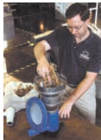
“Vortex” forage sample dryer is faster and easier than other methods used to determine moisture content, says Dennis Buckmaster, who designed the inexpensive, simple-to-build device.
