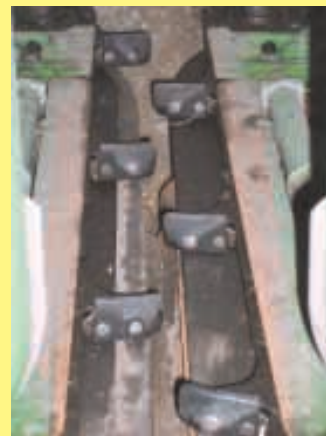
Plastic extenders on gathering chain paddles feed corn into combine more aggressively, reducing plug-ups.
