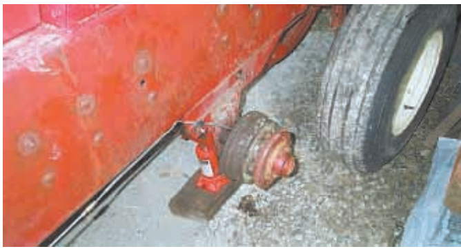
Ken Rakoz removed one of the wheels from his IH 435 baler and mounted this car brake drum on the wheel hub. Brake keeps baler from skidding on hillsides.
