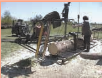
Don Fraser uses his home-built sawmill to make octagonal logs. Double-bladed saw cuts two sides of the log at a time.
