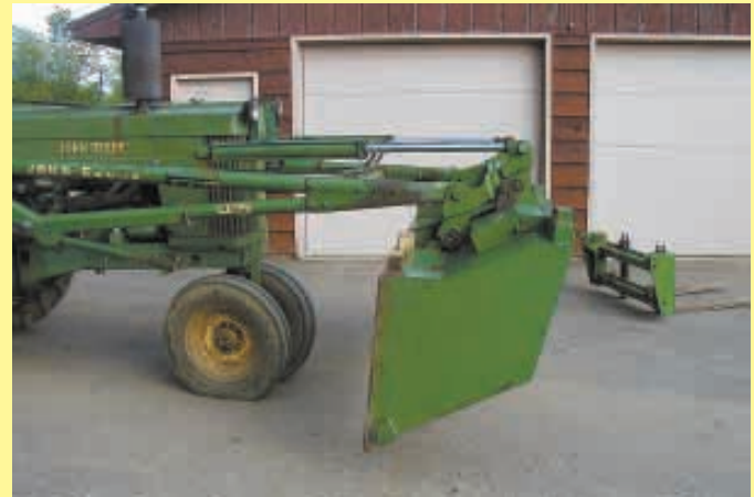
He reworked the hydraulic system on the tractor and added a beefed up loader. To get full use from the more powerful loader, he built a new 8-ft. bucket.
