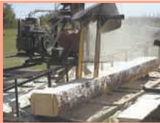
Don Fraser uses his home-built sawmill to make octagonal logs. Double-bladed saw cuts two sides of the log at a time.
