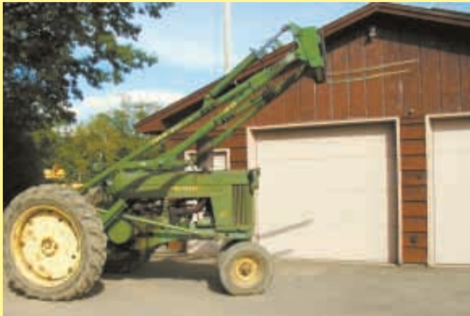
Tony Bunniss totally rebuilt the Deere 45 loader on his 1954 Deere 60 tractor. Quick-tach fittings make it easy to switch between a bucket and forklift.
